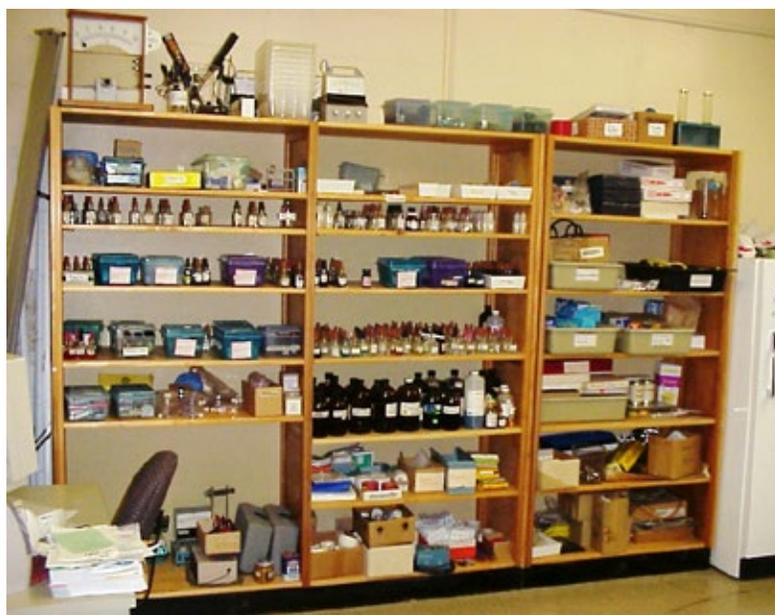
In this diagram, heavy objects can be seen on the top of the cupboards. Controlled products should be stored no higher than at eye level to reduce the chance of an accident.
